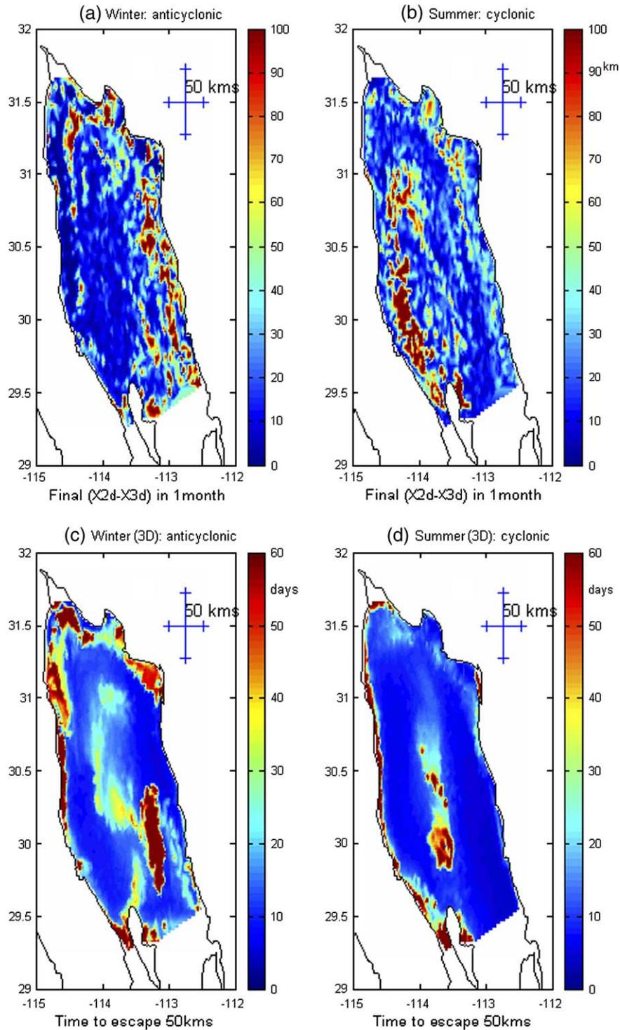
Fig. 4. Distance (km) between two particles released at each grid point, one with and one without vertical advection, after one month, for the (a) anticyclonic and (b) cyclonic gyre periods. Time to escape 50 km radius from the initial position, for the 3D case, for the anticyclonic (c) and cyclonic (d) gyre periods.
